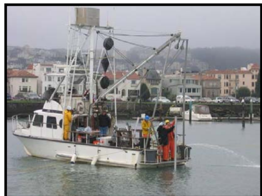
Vibracore sediment samples are collected for characterization of deposited materials to determine reuse and/or disposal options.
