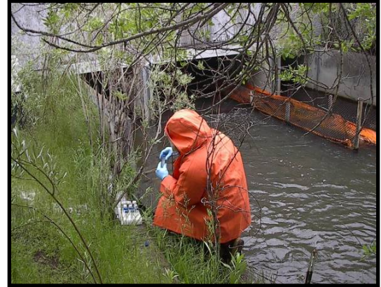
Grab sampling for volatile organic compounds to assess presence of petroleum based constituents in surface water.
