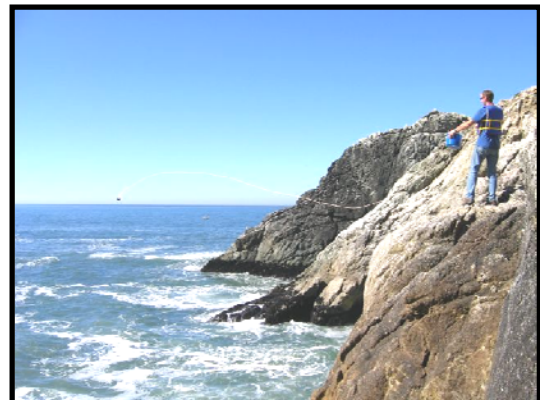
Shore-based water sampling data is used to model dye dilution in the receiving water.
