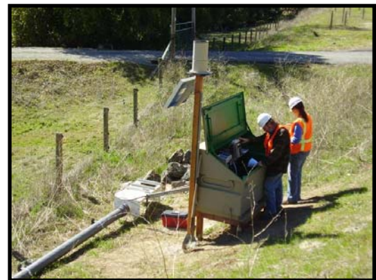
Specialized flow measurement and sampling station coupled with highly experienced staff to ensure valid BMP effectiveness testing.
